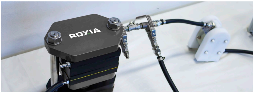
Filter press test unit simulates the operation of the full-size industrial filter.
