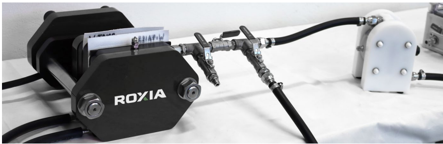
Filter press test unit simulates the operation of the full-size industrial filter.
