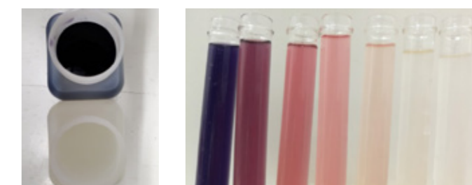
Roxia Plasma Oxidizer effectively removes colour from wastewater.
